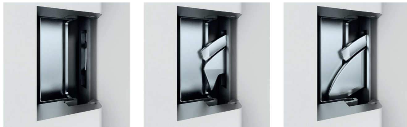
01+02 Door open: Weatherseal hook and hook retracted. Door closed: The weatherseal hook activates, the hook extends ... and engages deep into the keep rail.
